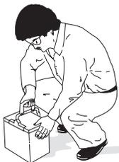
Batteries are heavy. Use proper lifting techniques when moving them. Always lift the battery with a commercially available battery lifting device. Do not tip batteries when removing or
